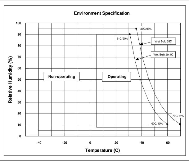
Figure 4 Limits of temperature and humidity
