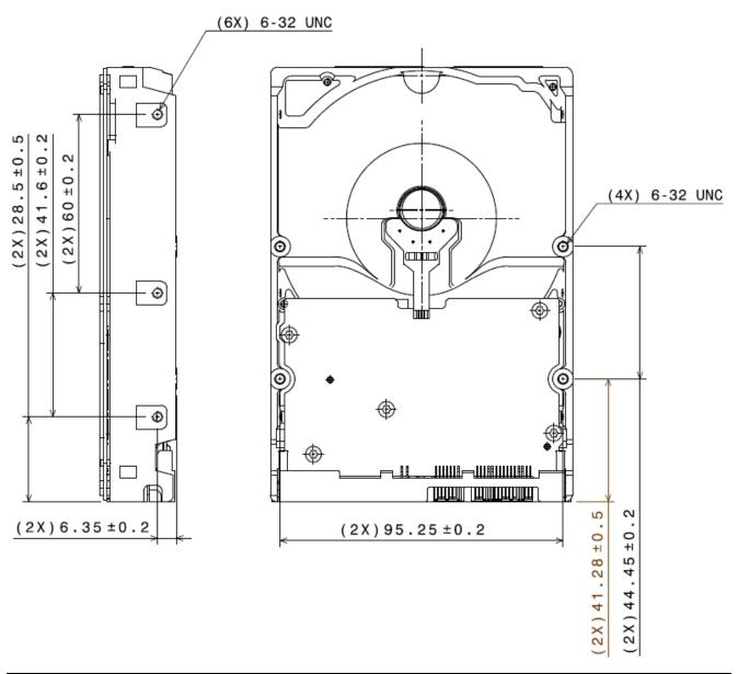
Figure 6 Bottom and side views with mounting hole locations
