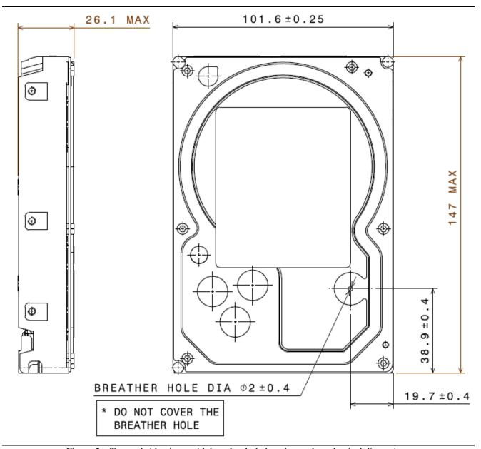
Figure 5 Top and side views with breather hole location and mechanical dimensions
