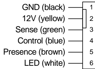
Figure 14: 6-Pin Cooling Fan Connector
