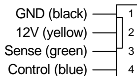
Figure 13: Cooling Fan Connector
