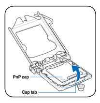
5. Position the CPU over the socket, ensuring that the gold triangle is on the bottom-left corner of the socket, and then fit the socket alignment keys into the CPU notches.
