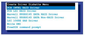
Use the arrow keys to select the type of RAID driver disk you want to create and press <Enter> to enter the sub-menu.
