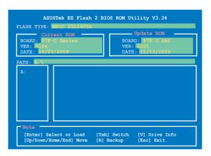
3. Press <Tab> to switch between drives until the correct BIOS file is found. When found, EZ Flash 2 performs the BIOS update process and automatically reboots the system when done.
