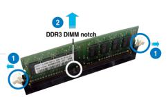
2. Remove the DIMM from the socket.
