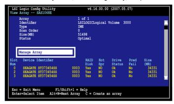
From the Manage Array screen select Manage Hot Spare, then press <Enter>.
