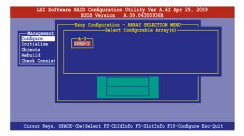
5. Press <F10> again, the virtual drive information appears including a **Virtual Drive** menu that allows you to change the virtual drive parameters.
