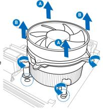
4. Carefully remove the heatsink and fan assembly from the motherboard.
