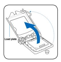
Remove the PnP cap from the CPU socket.
