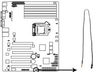
P7F-C Series Thermal sensor cable connector
