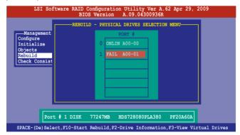
3. After selecting the drive to rebuild, press <F10>. When prompted, press <Y> to rebuild the drive.
