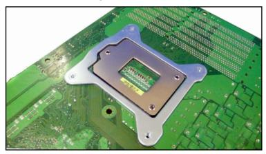
2. Use a Phillips screwdriver to tighten the four heatsink screws in a diagonal sequence.
