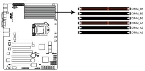
P7F-C Series 240-pin DDR3 DIMM sockets
